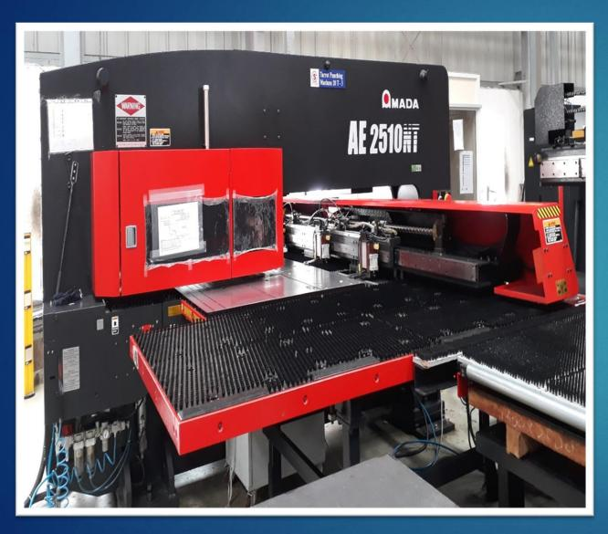
Amada Turret punching machine designed With Japanese technology capable  $\rho f_{o}$  processing 4ft X 8ft sheets, the AE-NT series has a large capacity turret to ensure stable, high speed, high-quality processing.
