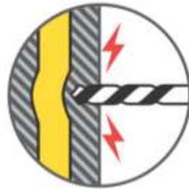
Mechanical damage of insulation
